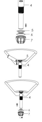
5. Close the drain and fill the sink with water. Check for leaks. If water is leaking from the drain, refer to steps 1-4 or tighten the area where the leak is occurring.
