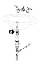
8 Connect supply line to faucet (finger tight) and carefully bend tubes to engage with the supply shut-off valves. Tighten connections at faucet and shut-off valves for secure seal.
