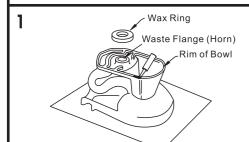
Insert the new toilet bolts in the slotted flange with the bolt heads down. Place the toilet bowl upside down on a soft material to prevent scratching. Place the wax ring evenly around the waste flange (horn), with tapered end of the ring facing the toilet. Apply a thin bead of sealant around the toilet base.
